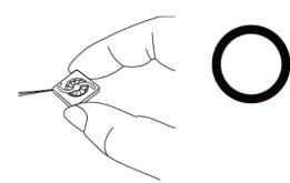
Don't pull fan with lead wires.
